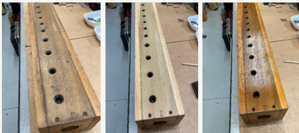
The pipe pneumatics of the Salicional Celeste offset chest with evidence of water damage and leather overlay technique.
