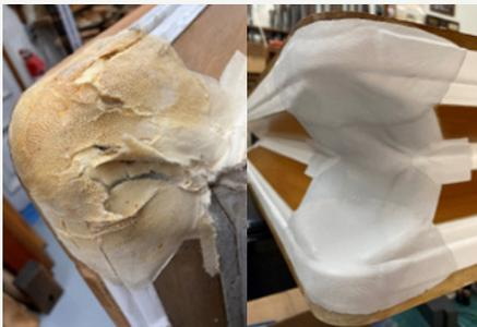
A compromised wind regulator rib due to incorrect glue usage that was newly made
